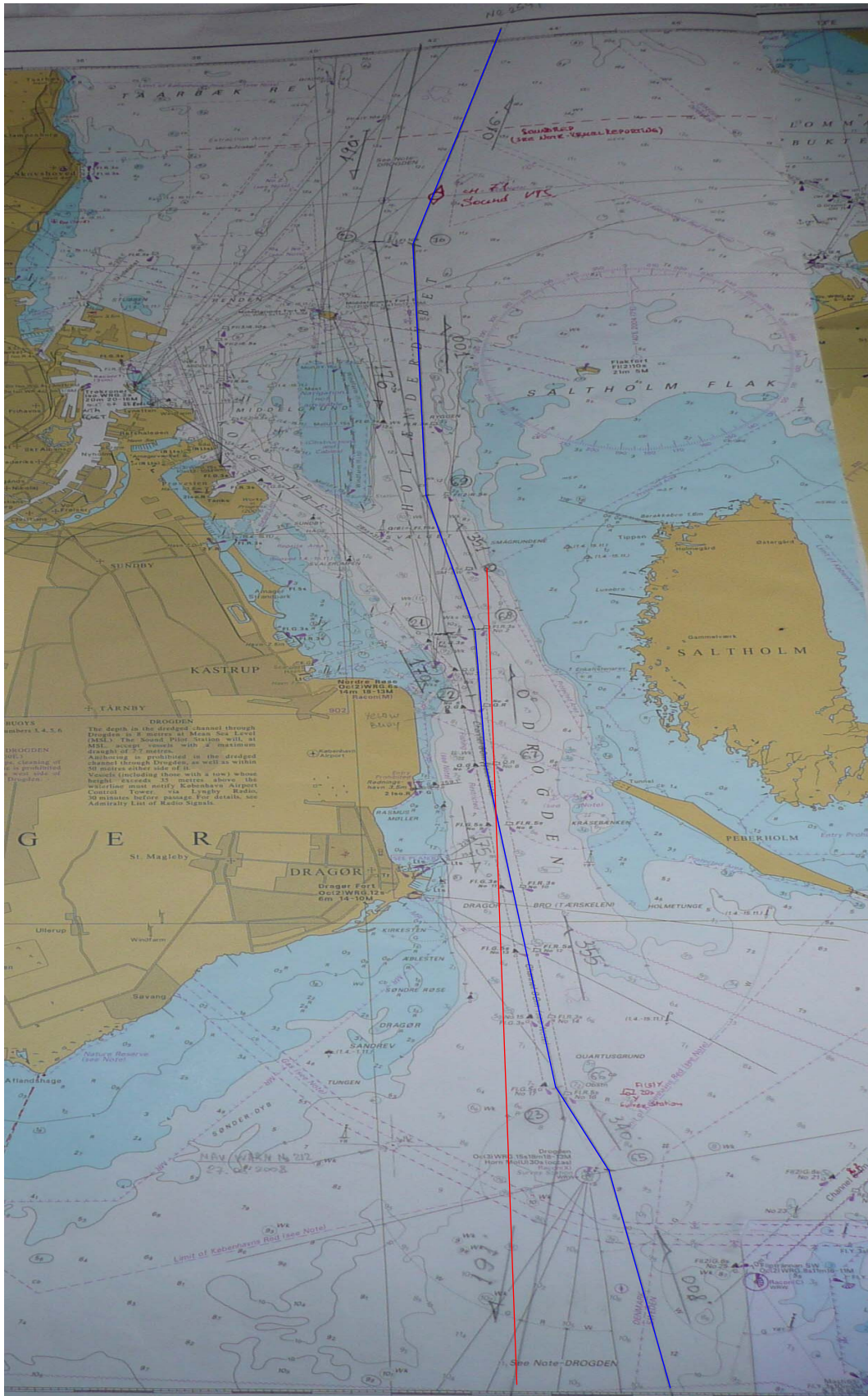
Photograph of KARIN SCHEPERS sea chart showing the planned track (blue line) and the track over ground (red line)
