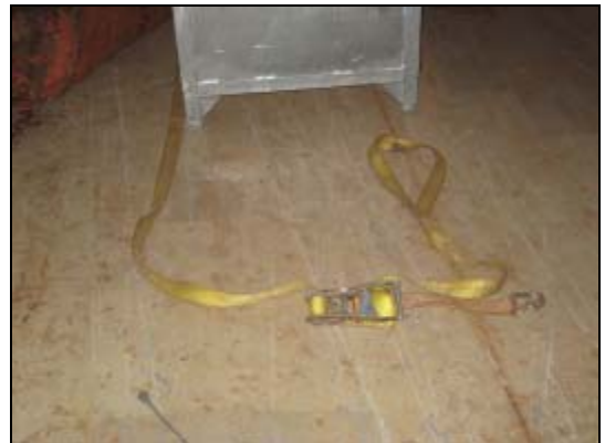
Web binder to secure the bins
