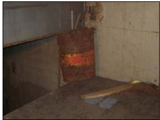
Drum caught between two sections of the tween deck
