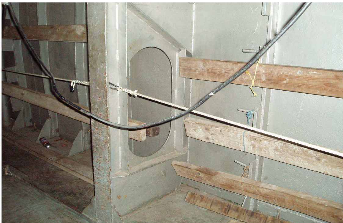
Passage way and web frame after mounting new ridge ropes with snap hooks
